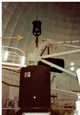
Figure 28a and b. The F/1 wide-field CCD camera being mounted at the Anglo-Australian telescope.
